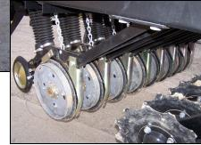
Model **FLXII88RD Rear Wheel Drive**. Three separate seed boxes. Plants almost any kind of grass, flower, or grain seed. 5.3 foot planting width with 8 inch spaced rows. Requires minimum 40 HP tractor.
